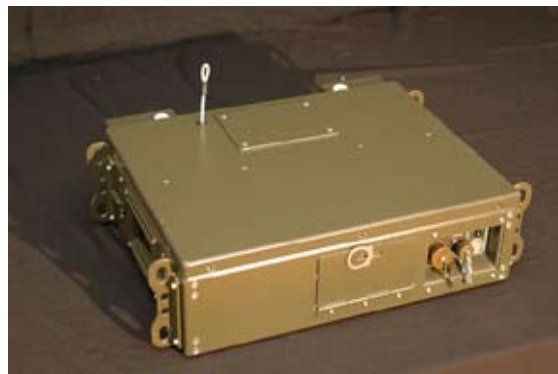
SPADES 300 Mk2 Guidance Unit (rear side with cable connectors, zeroize button and Mil-GPS bay)
